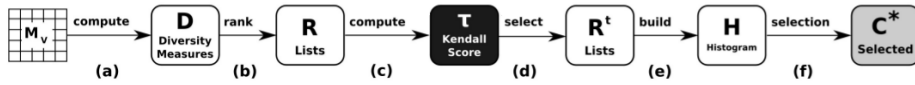
Fig. 3: The six steps for new classifier selection are: (a) Compute diversity measures from the validation matrix M_V ; (b) Sort \mathcal{R} lists by diversity measure scores; (c) Compute Kendall correlation coefficients among all ranked lists of classifiers \mathcal{R} ; (d) Select \mathcal{R}_{d_{H_1}} and \mathcal{R}_{d_{H_2}} or \mathcal{R}_{d_{L_1}} and \mathcal{R}_{d_{L_2}} ranked lists to be used in the next step; (e) \mathcal{R}^t lists with top t = 100 ; (f) Compute a histogram \mathcal{H} that counts the number of occurrences of each classifier; (g) Select the most appropriate classifiers |\mathcal{C}^*| based on their occurrence in \mathcal{H} and a defined threshold \mathcal{T} [12].
